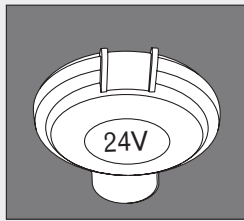
3. 24V Socket - For 24V output Location: At the bottom of the center console. Harness: Dashboard wiring harness
