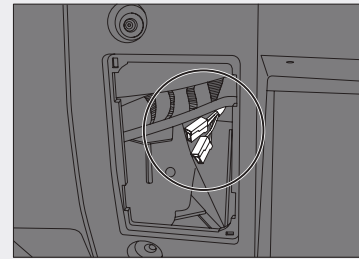
2. 24V Connector (2 nos) - For Electrical accessories Location: Left side of the steering column. Harness: Dashboard wiring harness
