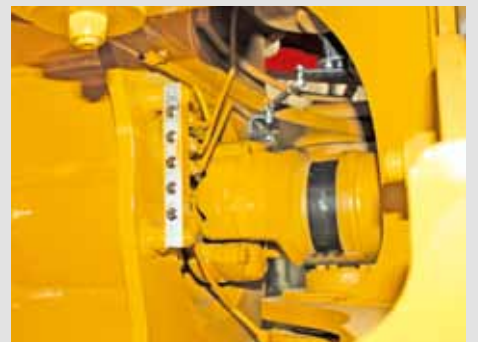
The centralised lube bank places difficult-to-reach nipples within reach. The convenient lube chart helps ensure that nothing gets overlooked.
