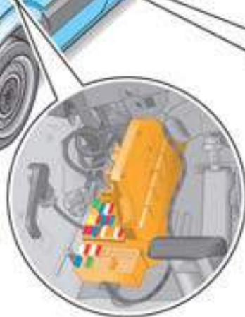
Onboard supply control unit J519, on the left A pillar
