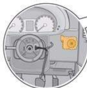
Electronic ignition lock D9, on the right next to the steering wheel
