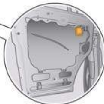
Driver door control unit J386, in the front left door
