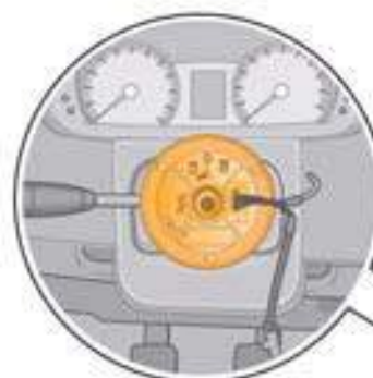
Steering column electronics control unit J527, on the steering column
