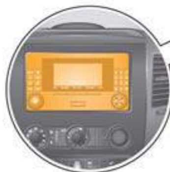
Control unit with display unit for radio and navigation J503/radio R, in centre of dash panel
