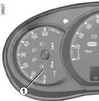
Rev counter 1 (graduations \times 1000 )
