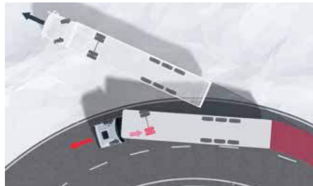
ESP compensatory braking when vehicle is understeered
