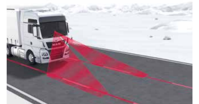
Lane Guard System (LGS) including Lane Return Assist (LRA)
