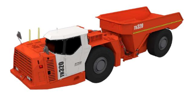
Sandvik TH320 is a narrow 20 metric tonne truck designed for small and medium-sized hard rock mines, fitting in a 3 x 3 meter heading. Despite the relatively high payload capacity, this underground truck has the same overall width as most 15-ton trucks on the market. As all Sandvik underground mining trucks, it is designed to operate fully loaded and at high speeds on long spiral haulage ways with up to 20% gradients.
