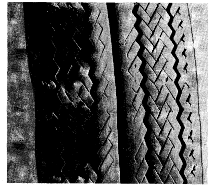
CUPPING—UNDERINFLATION AND/OR MECHANICAL IRREGULARITIES
