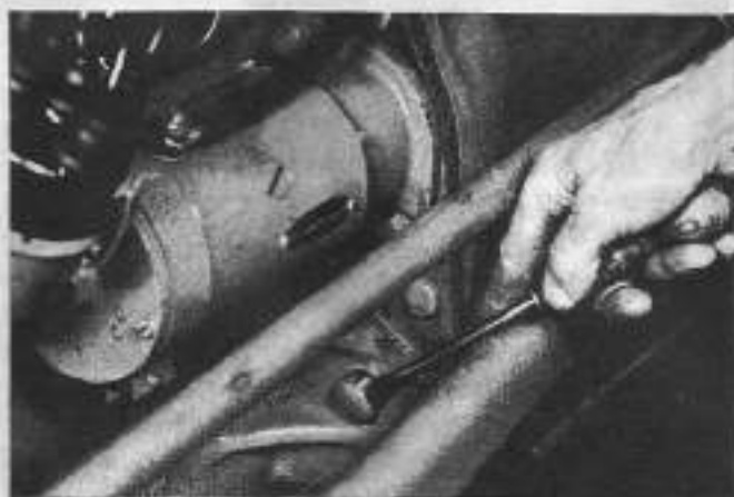
Removing timing hole button plug
