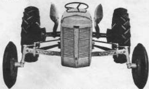
Wide tread width for row-crop operation.
