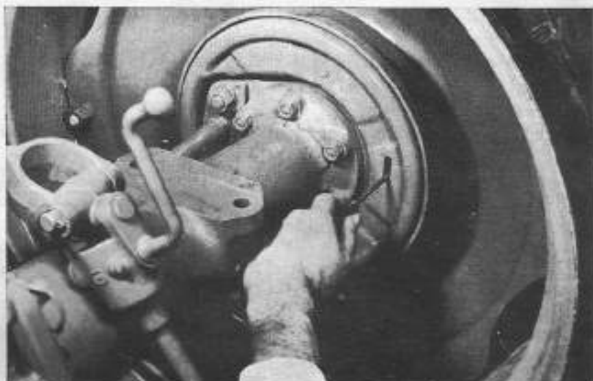
Adjusting brake shoe action on brake drum of rear wheel.
