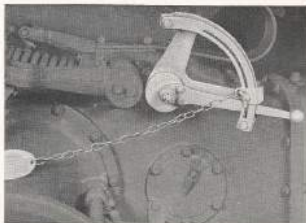
Finger-tip Control Lever locked down with Chain and Wedge Assembly.
