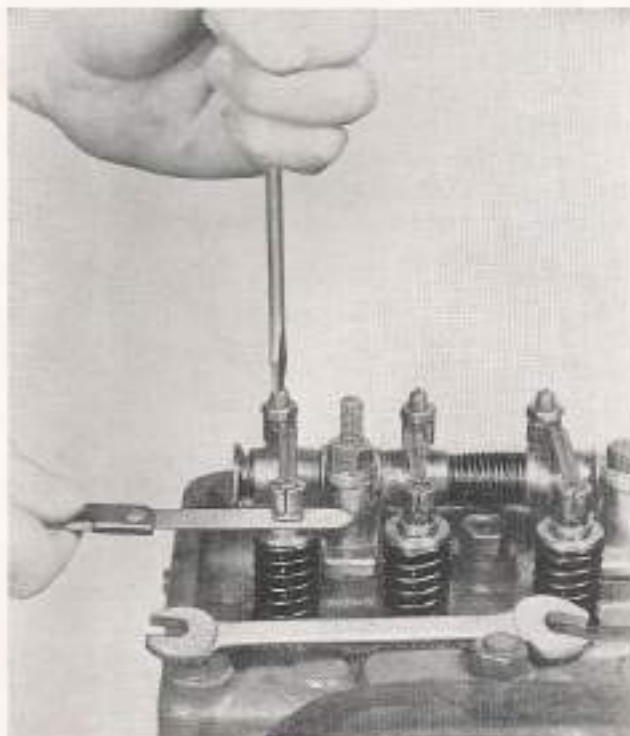
Adjusting the Valves.
