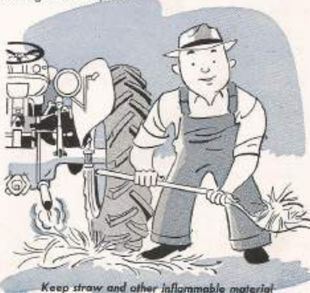
Keep straw and other inflammable material away from exhaust pipe to prevent fire.
