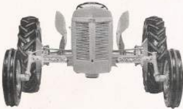
76' Wheel Spacing for row-crop work.
