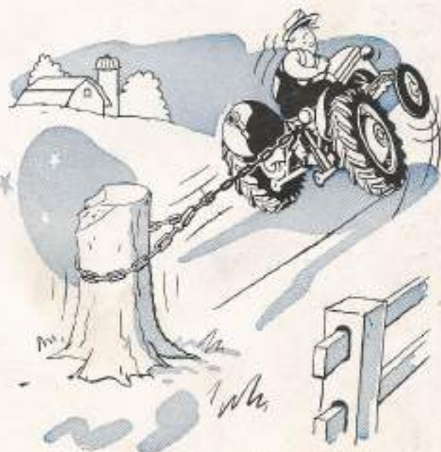
Never pull from upper link connection.
