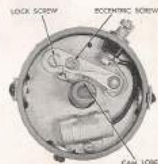
Distributor Points fully open.
