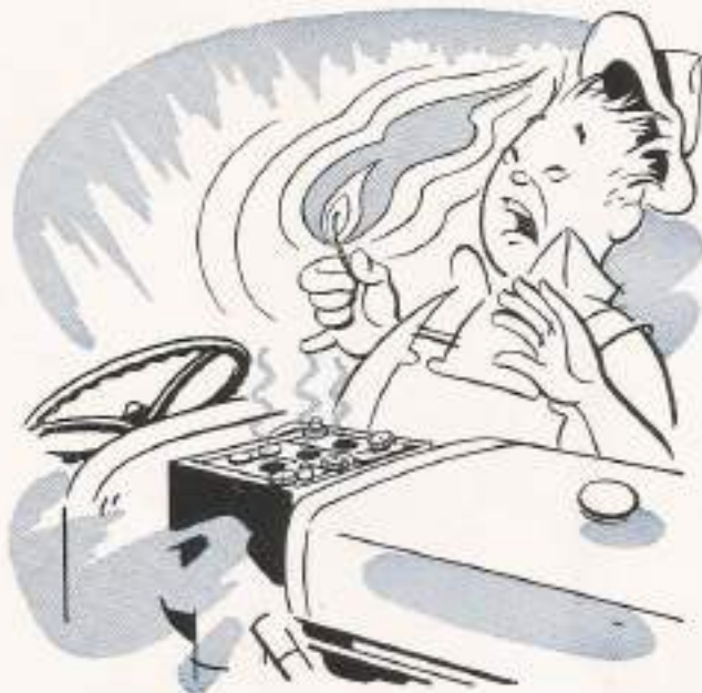
Keep flames away from battery filler cap openings.
