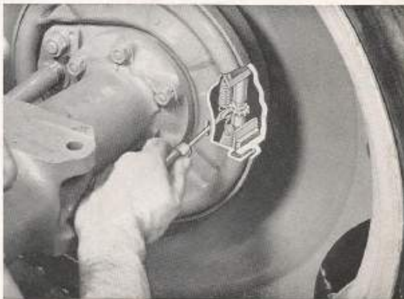
Adjusting Brake Shoes.
