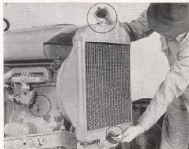
Open the two Drain Cocks and remove Pressure Cap when draining Radiator.
