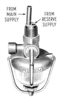
When tractor is to be idle for 30 days or more, drain the entire fuel system including the gasoline tank. Fuel should be removed through bottom of carburetor, with sediment bulb valve on "reserve." Gasoline, when stored, forms a gum or wax which has a tendency to clog up the small pores and openings in the carburetor. For the same reason, do not use gasoline which has been stored for more than 60 days.
