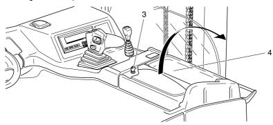
The drive current control system and the truck fuses are readily accessible for servicing purposes.
