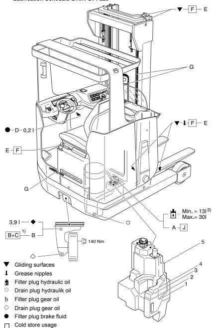
2) Filling amount see "Checking the hydraulics oil level"
