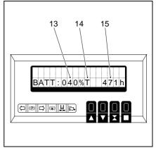
**Battery discharge monitor:** In case of undershooting the rest capacity the lifting function is disconnected. LISA indicates a corresponding message.
