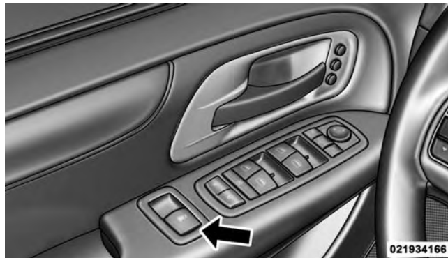
Power Vent Window Switch Open/Close
