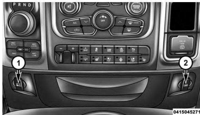
Power Outlets — Center Stack
