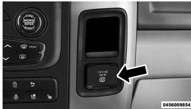
Power Inverter Outlet
