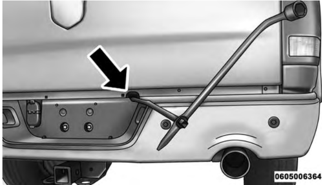
Inserting The Jack Extension Tube Into The Access Hole
