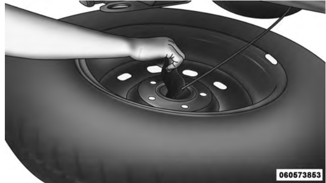
Reinstalling The Retainer
