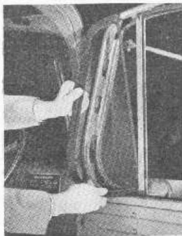
Fig. 63. Removing door fixed glass. (All models except Bus.)
