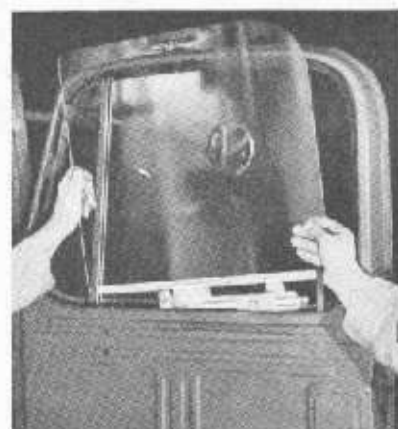
Fig. 62. Removing door drop glass. (All models except Bus.)
