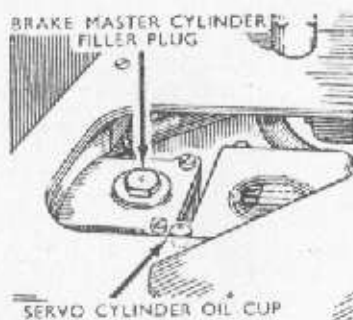
Fig. 7. Brake fluid reservoir and servo cylinder oil cup.
