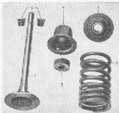
Fig. 39. Inlet valve details. 1. Valve spring cap. 2. Valve spring. 3. Valve stem oil seal felt. 4. Oil seal retainer. 5. Valve. 6. Valve retaining collars. When replacing the inlet valves, replace the valve in the head; then fit the felt seal on top of the valve guide, followed by the seal retainer, the valve spring—close coiling against the cylinder head—the valve cap and (with the spring compressed) the two tapered collars. The exhaust valves are assembled in the same way, except that no oil seal felt is used, and the seating washer is fitted under the spring instead of the oil seal retainer.
