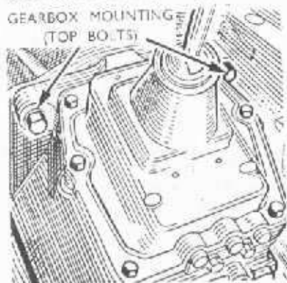
Fig. 28. Gearbox top mounting bolts.
