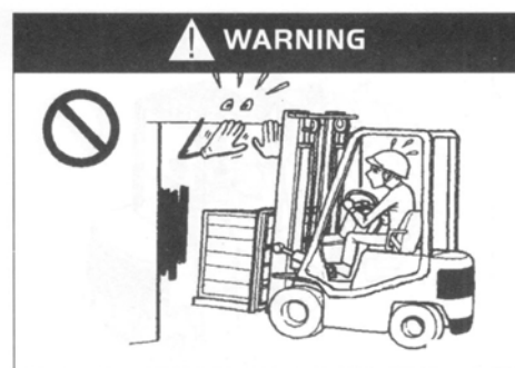
Notice Height Of Working Area At Any Time
