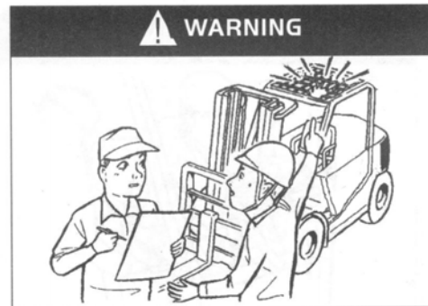
Do Not Drive Damaged Forklift
