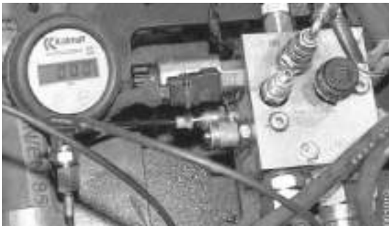
Pressure plate, gas pressure brake accumulators
