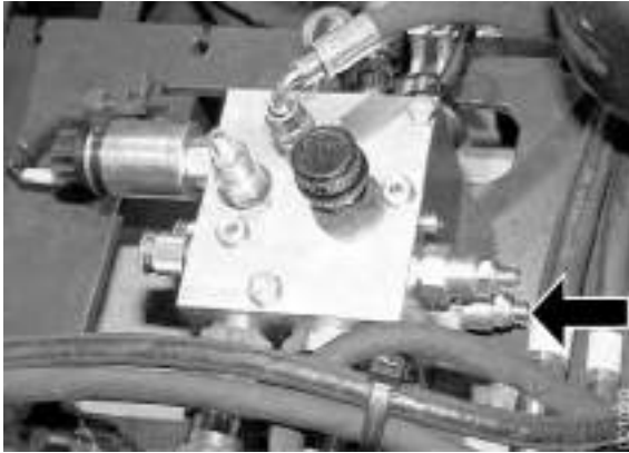
Adjusting screw accumulator charging pressure
