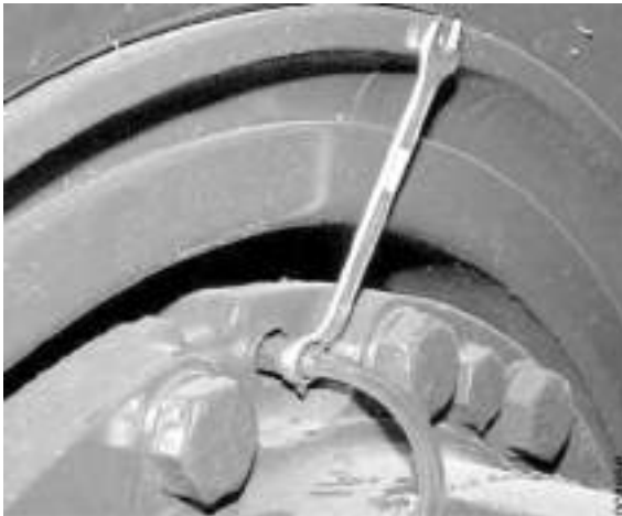
Bleed nipple, brake cylinder, on top of the drive axle at the wheel hub's inner short side (left-hand side).
