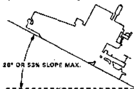
Slope Limitation for Engine Operation when Paver is Headed Uphill Figure 6
