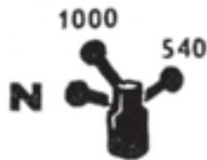
engaged with the control lever (Fig. 82) in such a way that the position to the left serves for 540 r.p.m., the position to the right is for 1.000 r.p.m., the forward position (in the driving direction) is neutral. The P.T.O.-shaft without changeable end pieces has only six-spline profile.
