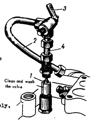
FIG.23. CLEANING AND WASHING CRANKCASE VENTILATION VALVE
