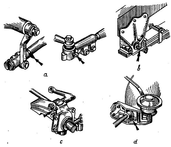
FIG.17. LUBRICATING POINTS FOR YC-1 GREASE (PRESS SOLID OIL), PRESS SOLID OIL "C" ' OR SOLID OIL "C" '
