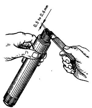
FIG. 12. MEASURING SPARK GAP
