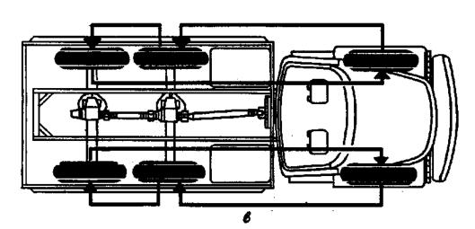
FIG.28. TYRE ROTATION DIAGRAM
