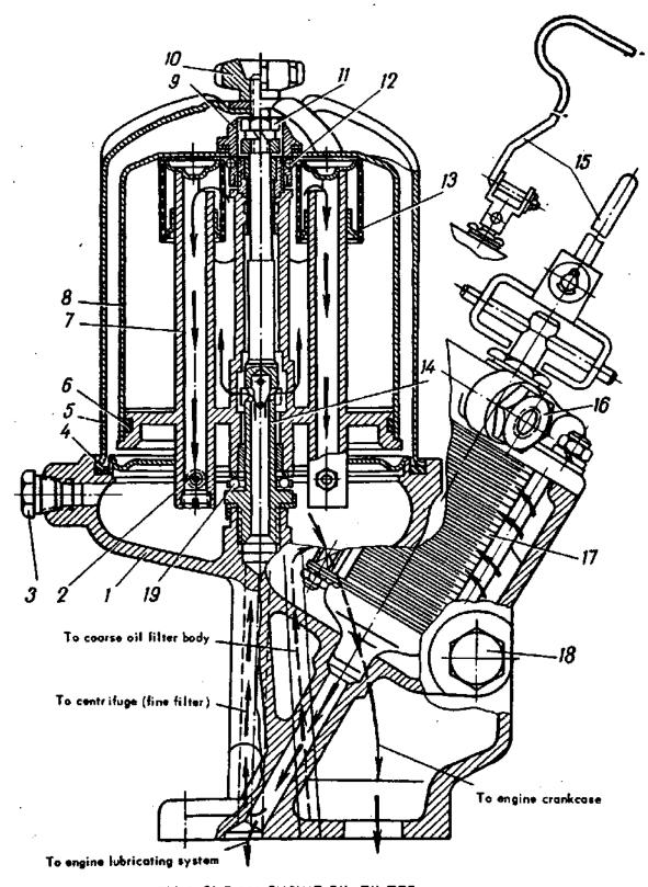
FIG.8. 3NJI-131 ENGINE OIL FILTER
