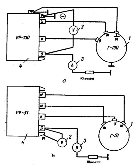
FIG.64. CURRENT REGULATOR AND VOLTAGE REGULATOR TESTING DIAGRAM
