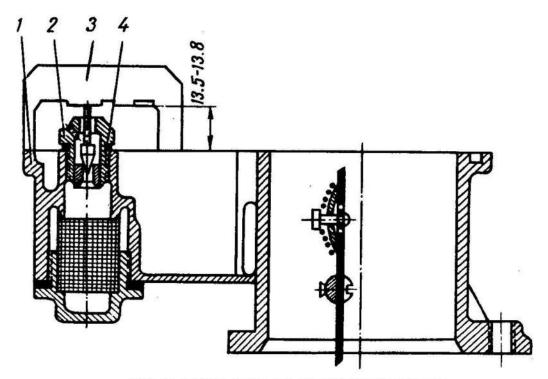
FIG. 60. NEEDLE VALVE ADJUSTMENT CHECK
