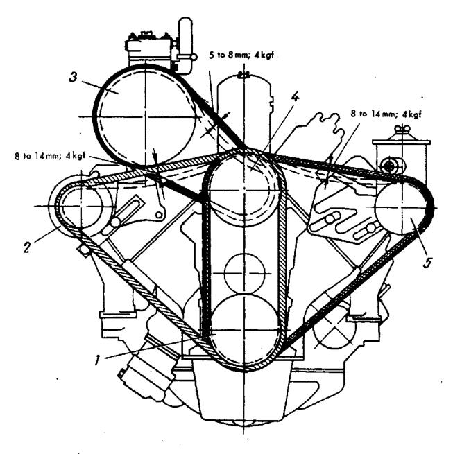
FIG.6. DRIVE BELT TENSION DIAGRAM
