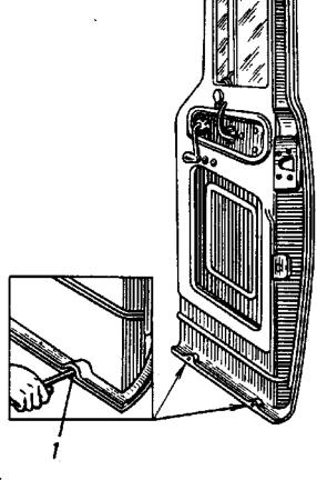
FIG.36. CLEANING METHOD FOR DRAIN HOLES 1 IN CAB DOORS
