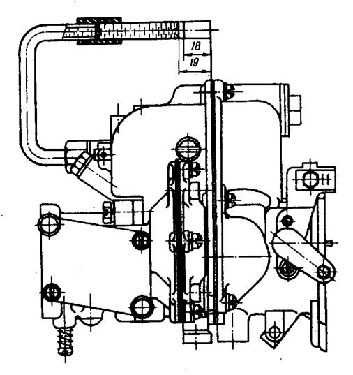
FIG.62, CHECKING FUEL LEVEL IN CARBURETTOR FLOAT CHAMBER WITH THE AID OF GLASS TUBE
