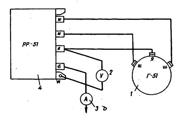
FIG.63. CUT-OUT RELAY TESTING DIAGRAM
