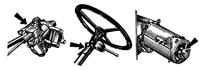
FIG. 35, LUBRICATING POINTS FOR 158 OR HNATHM-201 GREASE
