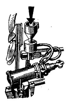
FIG. 19. LUBRICATING POINT FOR "P" OIL USED IN AUTOMOTIVE HYDRAULIC SYSTEMS (SUBSTITUTE IS TURBINE OIL 22 OR INDUSTRIAL OIL 20)
