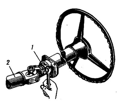
FIG.14. STEERING WHEEL END PLAY ADJUSTMENT
