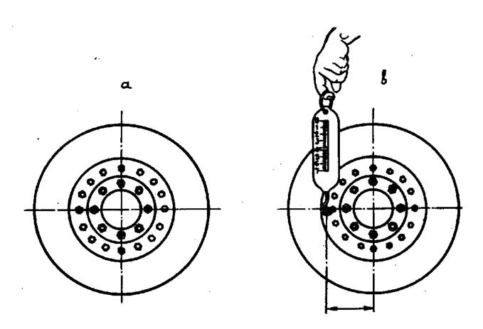
FIG.51. WHEEL BALANCING CHECK
