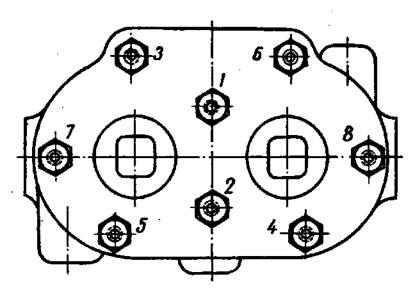
FIG.15. SEQUENCE OF TIGHT ENING NUTS OF COMPRESSOR CYLINDER HEAD STUDS
