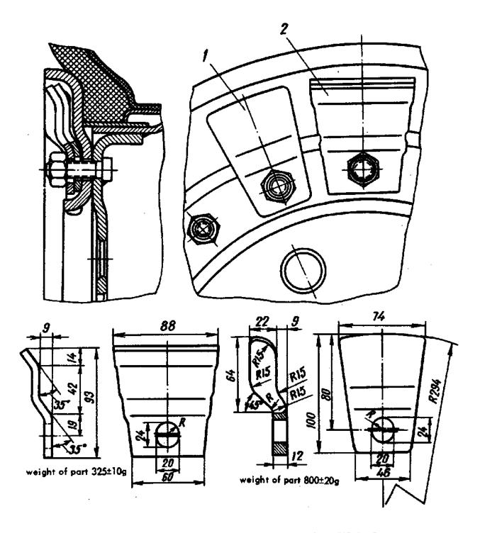
FIG.52. FITTING BALANCING WEIGHTS AND THEIR SIZES
