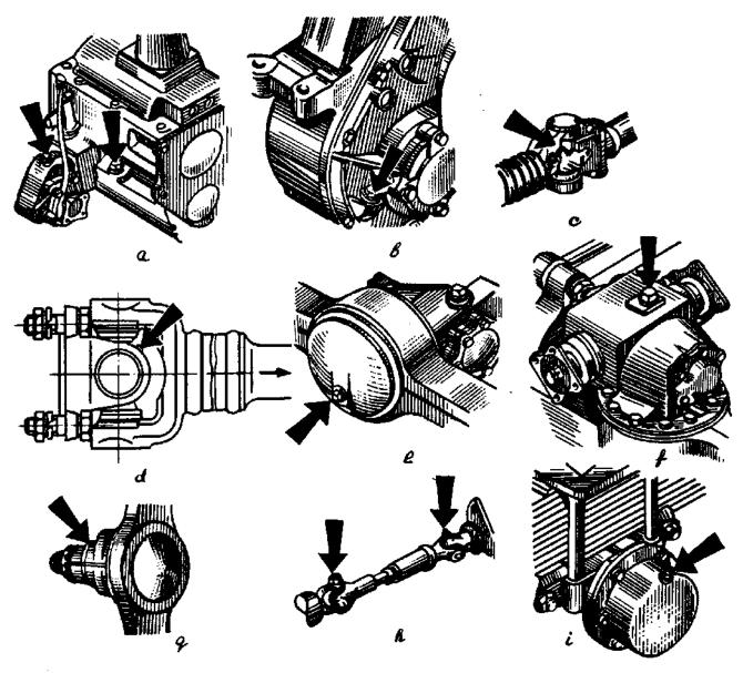
FIG. 18. LUBRICATING POINTS FOR T-146 AUTOMOTIVE TRANSMISSION OIL (WITH ADDITIVE)
