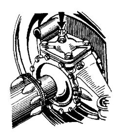
FIG.34. LUBRICATING POINT FOR AM LUBRICANT USED IN FRONT AXLE SHAFT JOINT AND KING PIN BEARINGS OF 31/11-131 TRUCK
