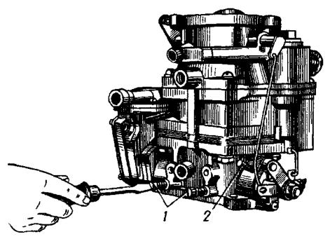
FIG.38. CARBURE TOR IDLE SPEED ADJUSTMENT
