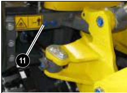
Fig. 49: Lubrication points of ball bearing race
