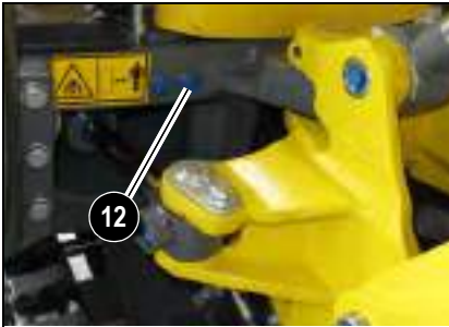
Fig. 51: Teeth lubrication point
