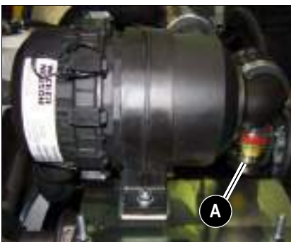
Fig. 19: Indicator for air filter contamination
