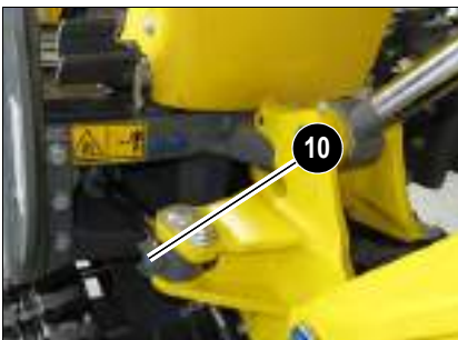
Fig. 48: Lubrication point on swiveling cylinder (swiveling console)
