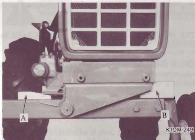
Blocking the front end of the tractor.
