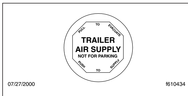
Fig. 5.3, Trailer Air Supply Knob
