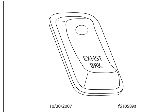
Fig. 5.7, Exhaust Brake Switch
