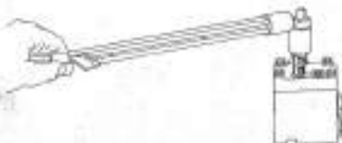
Fig. 28 - Tightening lowering valve loading
