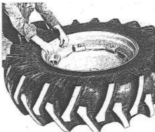
Fig. 13 — Taking out valve internals
