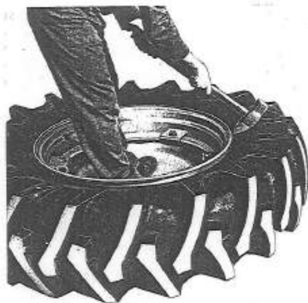
Fig. 14 — Loosening heel from rim flange
