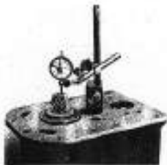
Fig. 29 - Checking level gear axial adjustment
