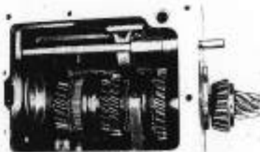
Fig. 28 - Assembling main shaft
