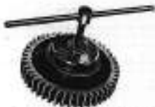
Fig. 9 - Extracting reducer wheel bearing
