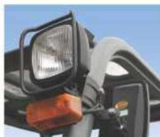
Protective light guards prevents damage
