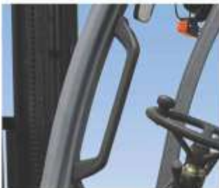
Large operator hand assisted access grip
