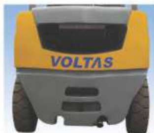
Large opening on counter weight for effective engine cooling
