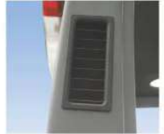
Top air inlet through canopy for cleaner air to engine
