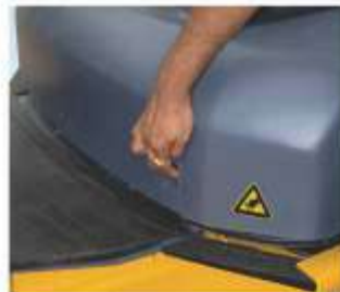
Lever for smooth opening of engine hood
