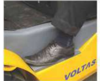
Wider operator foot rest for safer entry & exit
