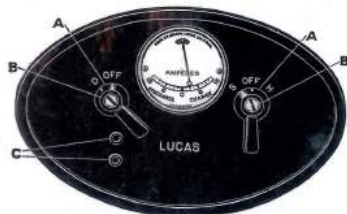
Fig. 5. View of switchbox. A—Switch levers. B—Securing screws. C—Inspection lamp plug adapter.
