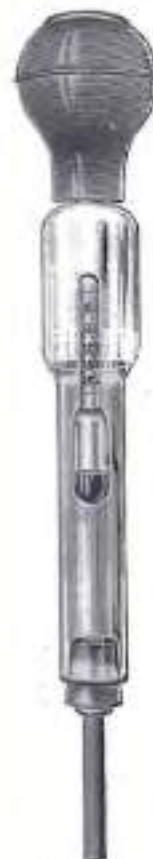
A Hydrometer, used for testing the state of the battery.
