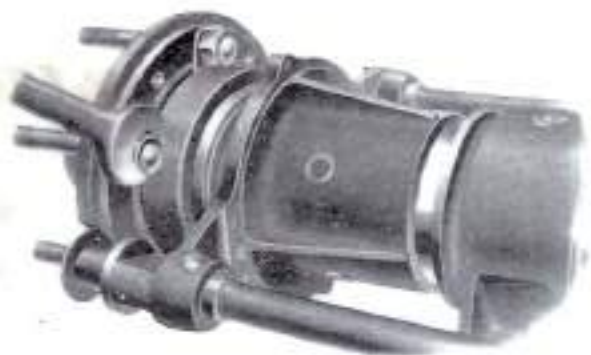
The new type of hub design in which it is not necessary to use any special tools for the removal of the hub and brake drum.
