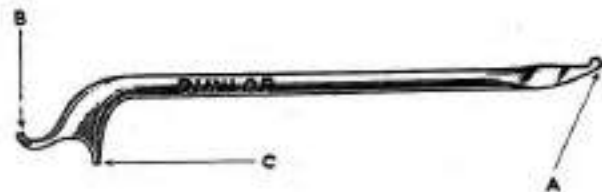
Fig. 1. The special tyre lever used for the fitting and removal of straight side cord tyres.
