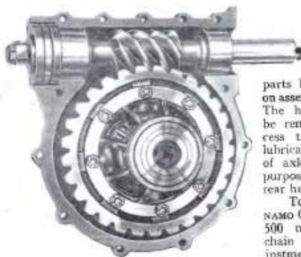
The construction of the Morris back axle worm drive and differential.
