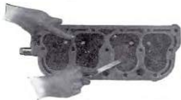
Scraping carbon from the cylinder head after it has been removed.
