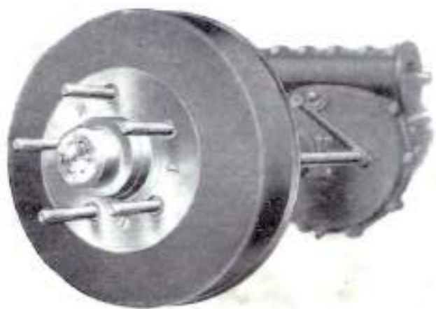
Showing the three counter sunk locking screws which hold the brake drum in position.
