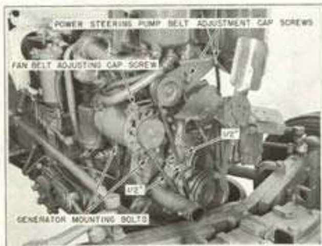
Figure 8-4 Power Steering Pump Belt Adjustment
