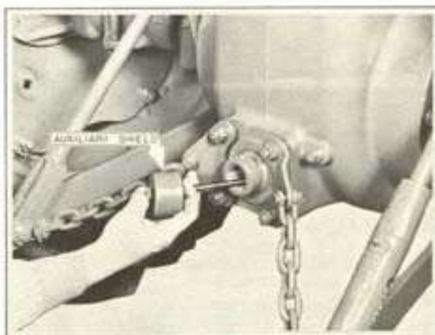
Figure 10-4 Installing Power Take-Off Auxiliary Shield
