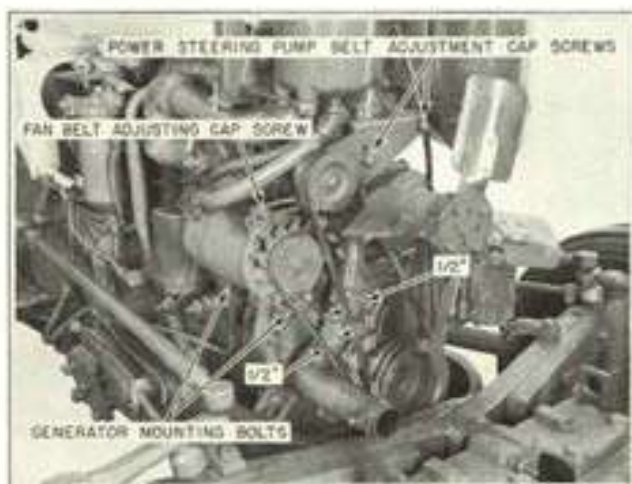
Figure 5-5 Fan Belt Adjustment
