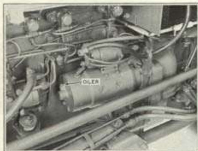
Figure 4-11 Diesel Starting Motor Lubrication
