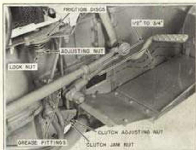
Figure 6-1 Clutch Pedal Adjustment
