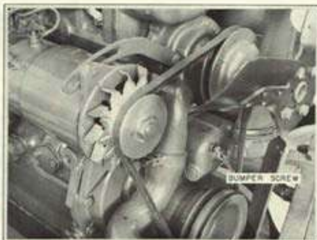
Figure 3-8 Governor Bumper Screw Adjustment
