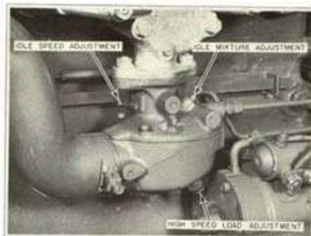
Figure 3-5 Carburetor Adjustments
