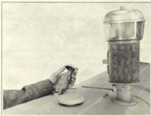
Figure 8-2 Checking Pump Reservoir Oil Level
