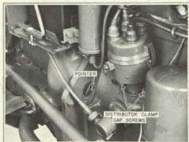
Figure 4-10 Timing The Ignition
