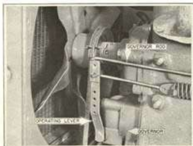
Figure 3-6 Governor Linkage Adjustment
