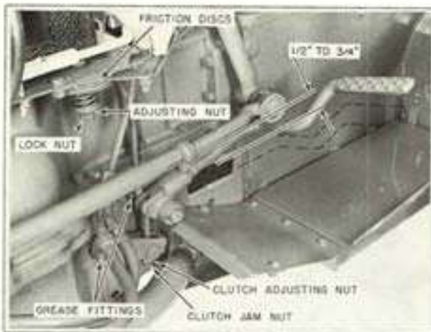
Figure 1-7 Clutch Pedal And Governor Control Friction Discs
