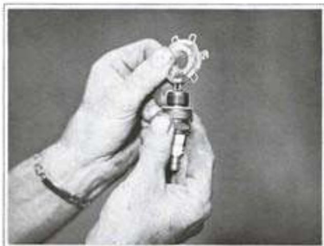
Figure 4-6 Checking Spark Plug Gap
