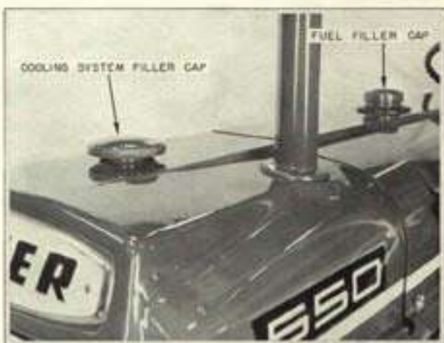
Figure 1-14 Radiator And Fuel Tank Filler Openings
