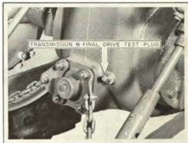
Figure 7-1 Transmission And Final Drive Test Plug
