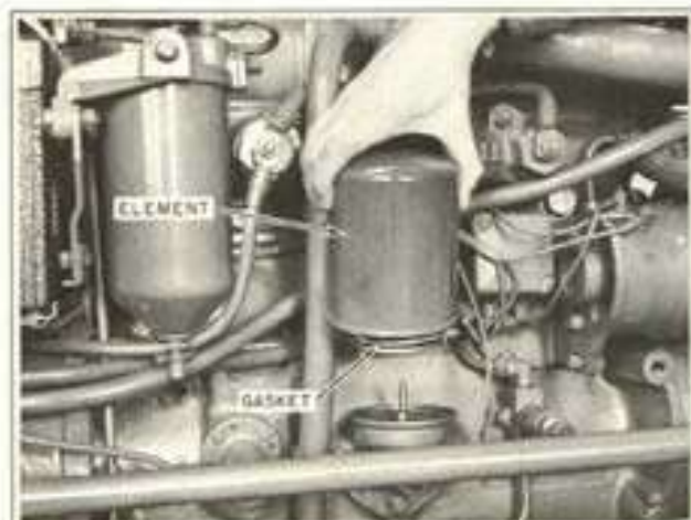
Figure 2-2 Servicing Oil Filter
