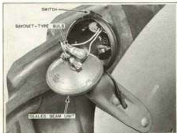
Figure 4-15 Servicing Combination Lamp
