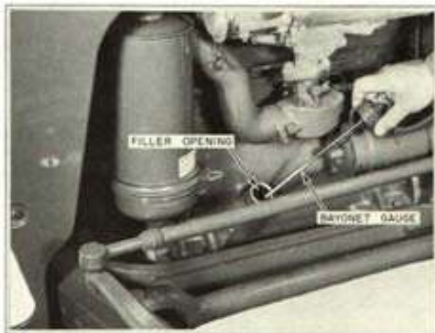
Figure 2-1 Checking Crankcase Oil Level
