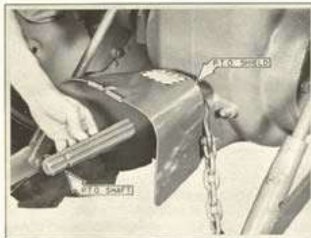
Figure 10-3 Installing Power Take-Off Shaft
