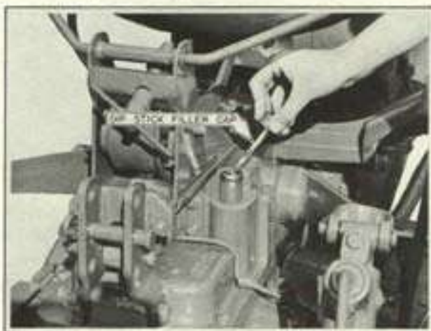
Figure 10-15 Checking Hydraulic Oil Level
