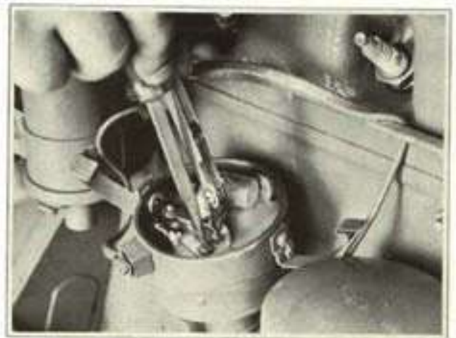
Figure 4-9 Adjusting Distributor Points
