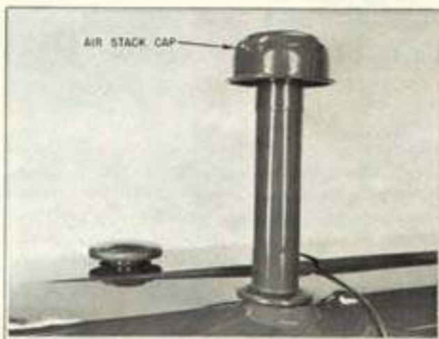
Figure 3-1 Air Stack Cap
