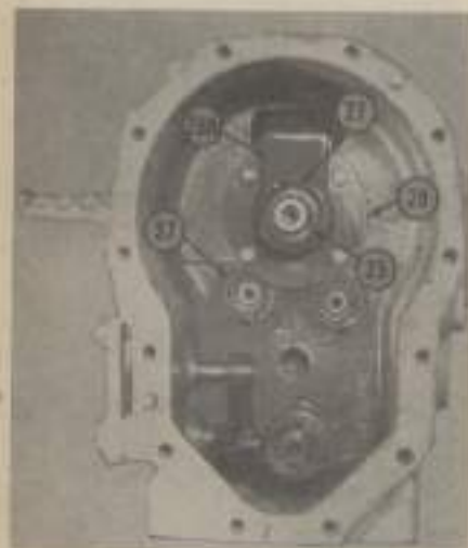
Fig. 103—View of D-14 and D-15 "Power-Director" compartment. After the snap ring (27) and the transfer tube (28A) retaining cup screws are removed, the outer (hollow) "Power-Director" clutch shaft (25), oil transfer tube (28A) and retainer (28) can be lifted out.
