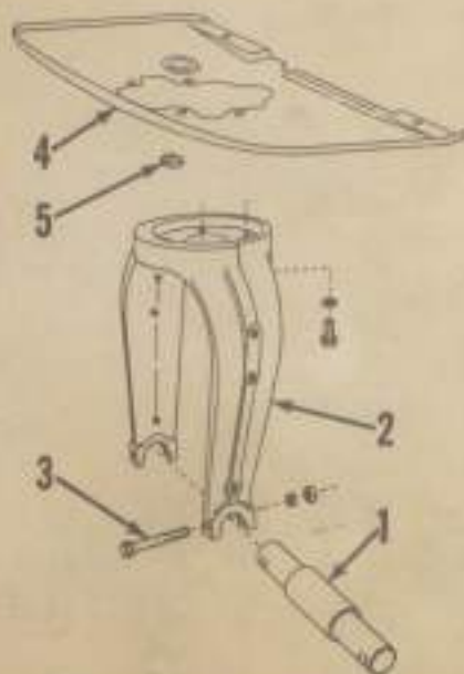
Fig. 1—Exploded view of single front wheel fork and associated parts.
