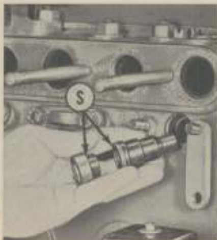
Fig. 79 — Installing the energy cell. If the surfaces (S) are rough or pitted, they can be reconditioned by lapping.
