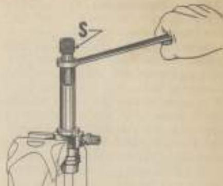
Fig. 74—Using Bosch tool (S) to center the nozzle tip while tightening the cap nut. Late production nozzles do not require the use of a centering sleeve.
