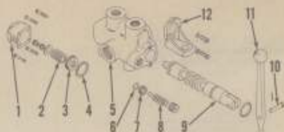
Fig. 167 — Exploded view of single-spool four-way control valve for operation of low-pressure double acting remote ram (available as optional equipment).
