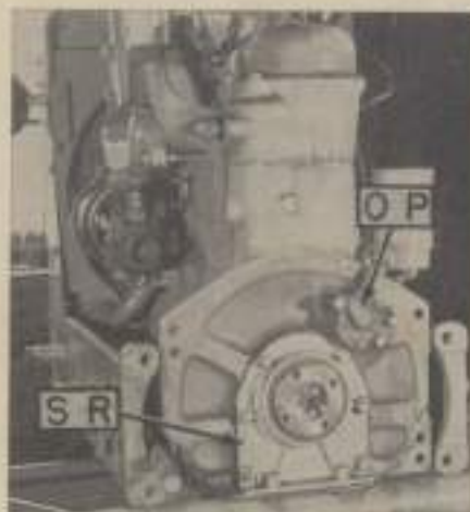
Fig. 50—On D-14 and D-15 non-diesel models, the crankshaft rear oil seal is contained in the seal retainer (SR). Oil pump (OP) can be removed after removing the flywheel.
