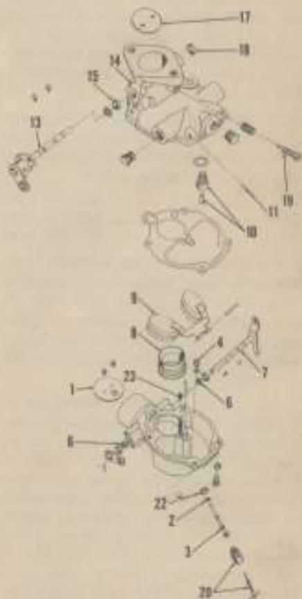
Fig. 60—Exploded view of Zenith carburetor used on some D-17 models. Refer to Fig. 58 for legend. Well vent jet is shown at (22).
