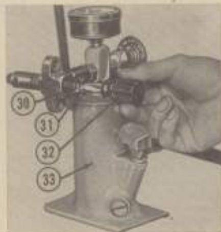
Fig. 71—Adjusting nozzle opening pressure, using a nozzle tester.
