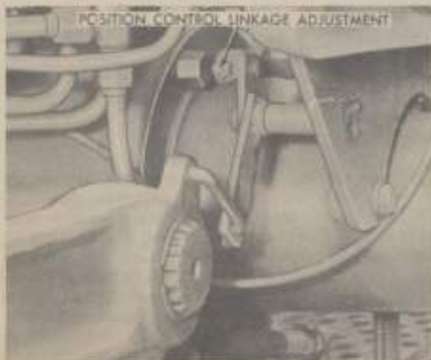
Fig. 175—View of position control linkage adjustment nut. Refer to paragraph 261 for adjustment procedure. Nut is self locking.
