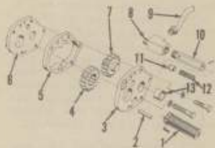
Fig. 111—Exploded view of "Power-Director" oil pump used on late production D-15 models.
