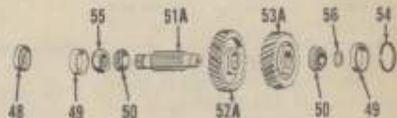
Fig. 108 — Exploded view of intermediate shaft and gears used on D-17 tractors after tractor Serial No. D17-24001.
