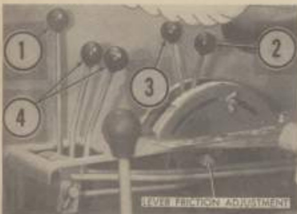
Fig. 173—View of Series IV D-17 hydraulic control levers and control lever friction adjustment nut.
