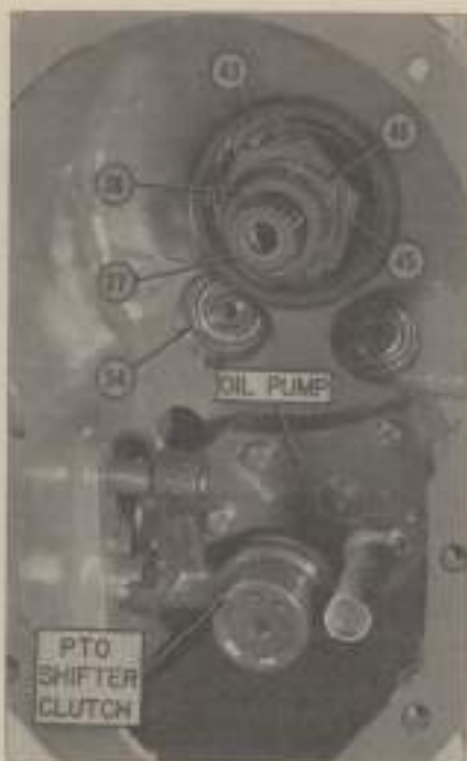
Fig. 105—View into D-17 "Power-Director" compartment showing the inner clutch shaft (27) and the outer (hollow) shaft (36).
