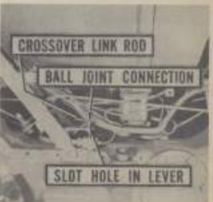
Fig. 159 — View of adjustment points for early type "lift-lower" linkage. Refer to paragraph 243.
