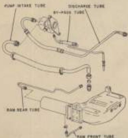
Fig. 13—Drawing showing the positions of the various power steering tubes used on all D-15 diesel tractors and D-17 diesel models prior to tractor Serial No. D17-38964.
