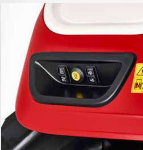
External actuation for rear PTO, rear hitch and a control unit for each of the rear mudguards.
