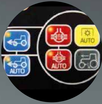
Automatic all-wheel drive and differential lock management
