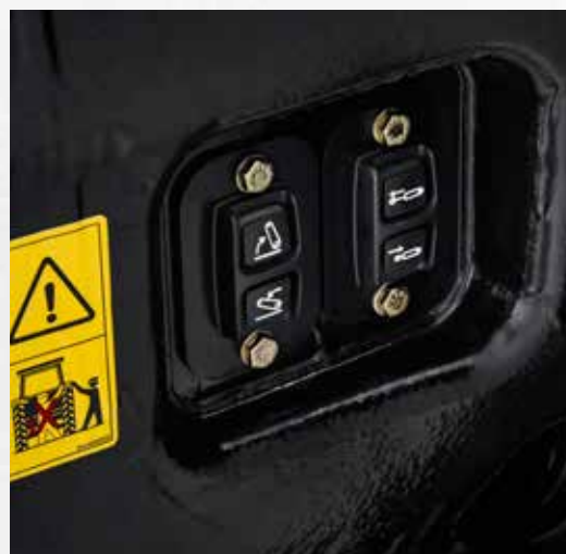
Easy to reach: External actuation of front hitch, front PTO and front control unit.
