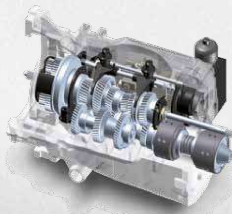
Continuously variable transmission from 0 to 50 km/h.
