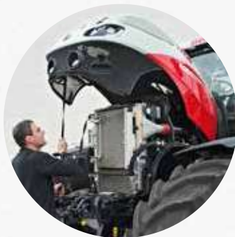
One-section bonnet support by gas struts can be lifted into two positions (45°/90°), even with a front-mounted attachment.
