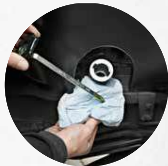
Checking of oil level and topping up without lifting the bonnet
