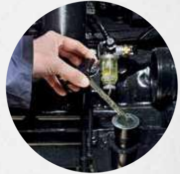
Checking of oil level and topping up without lifting the bonnet
