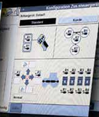
Define buttons to ctuate the control units
