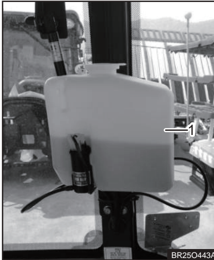
(1) Wash Liquid Tank
