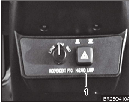
(1) Emergency Lamp Switch
