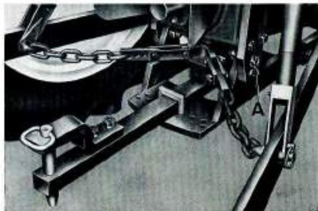
FIGURE 1/22. DRAWBAR IN EXTENDED POSITION
