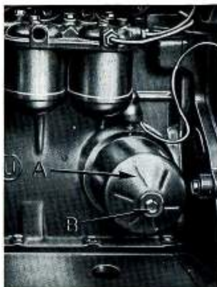
FIGURE 3/21. ENGINE OIL FILTER A. Filter body B. Securing bolt
