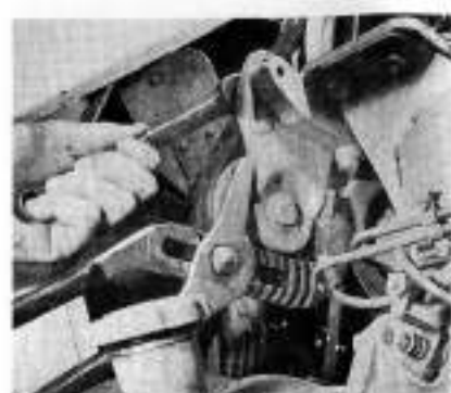
Turn the adjusting bracket until the correct belt tension is reached. Then tighten the bolt.
