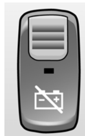
The safety switch for the battery master switch is located on the instrument panel.
