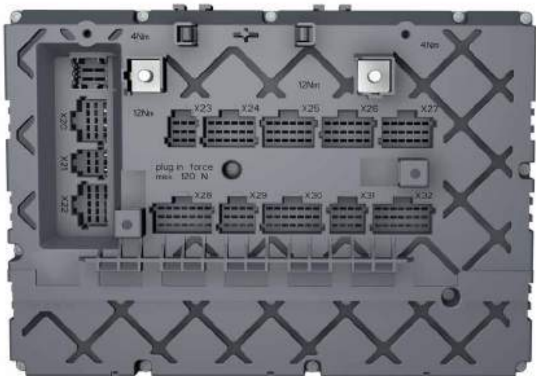
View of rear section of SSAM
