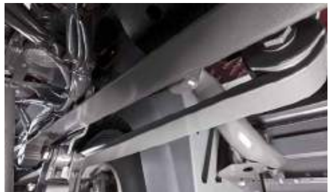
Rear spring, 5.0 t, parabolic, 1-leaf (Q2N)
