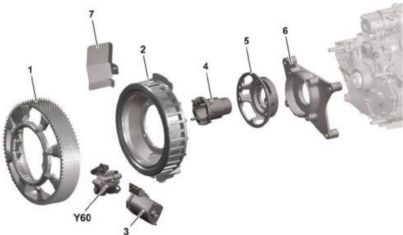
Permanent magnet retarder (B3G) on transmission G 90-6
