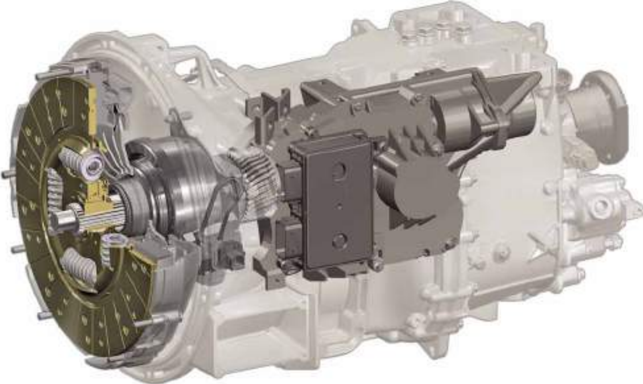
Clutch for Mercedes PowerShift 3 (G5G)
