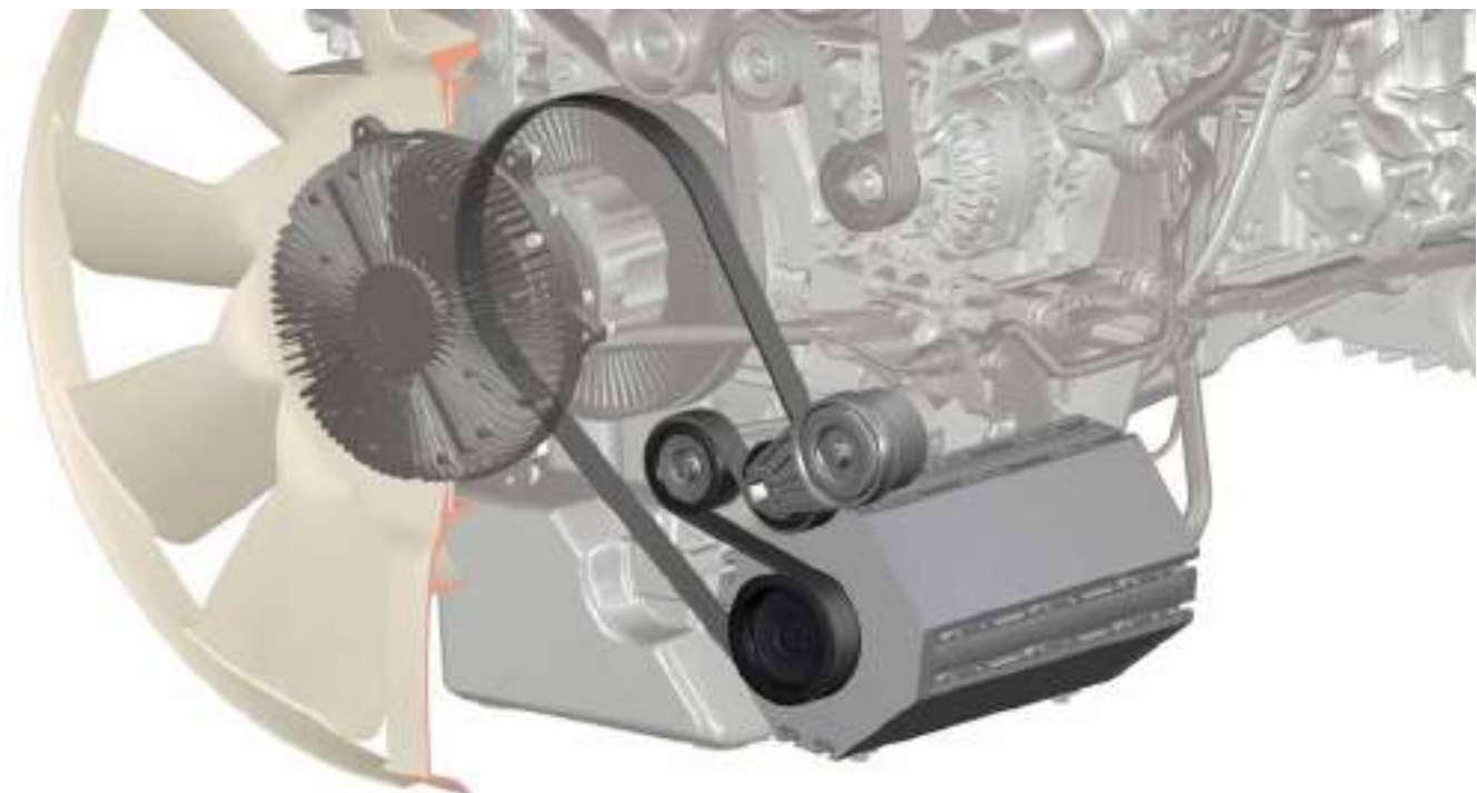
Engine power take-off, Frigo alternator AW 22,5
