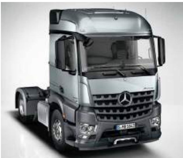
StreamSpace L cab, body floor height 600 mm
