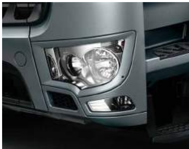
Halogen headlamp with front fog lamp (L1H)
