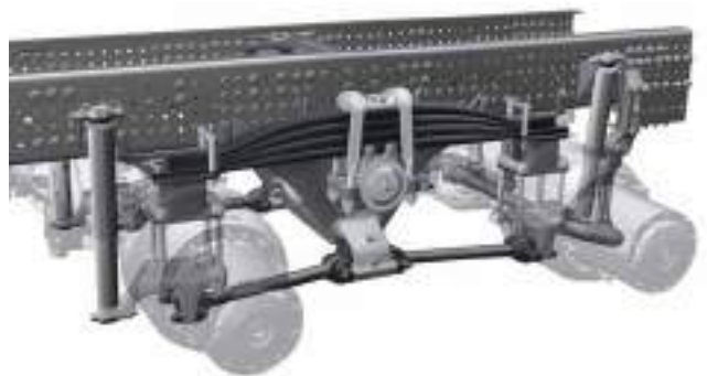
Steel suspension with 2 driven rear axles
