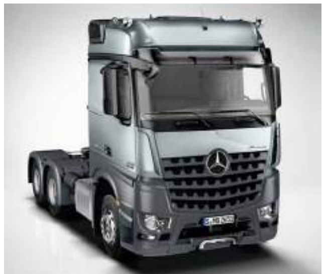
BigSpace L cab, body floor height 765 mm
