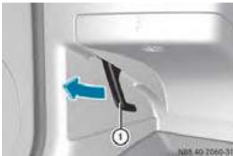
Hood release lever in the driver's footwell
