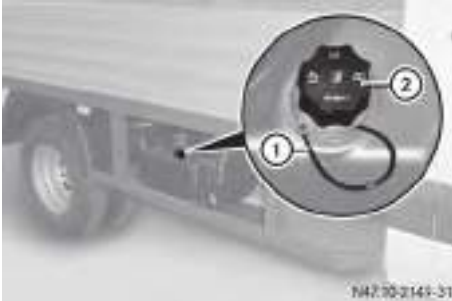
DEF tank on the right-hand side of the vehicle (example: Chassis Cab)
