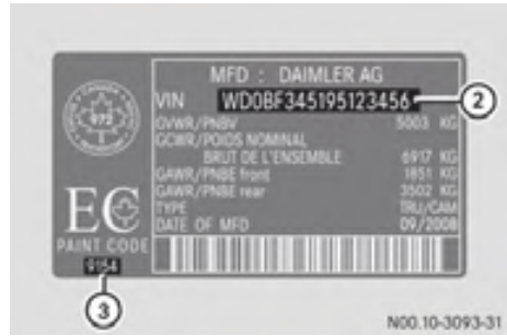
Example of a vehicle identification plate (vehicles for Canada)
