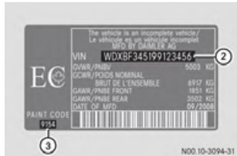
Example of a chassis identification plate (vehicles for Canada)
