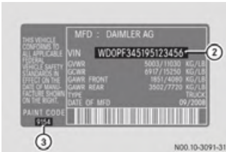
Example of a vehicle identification plate (US vehicles)
