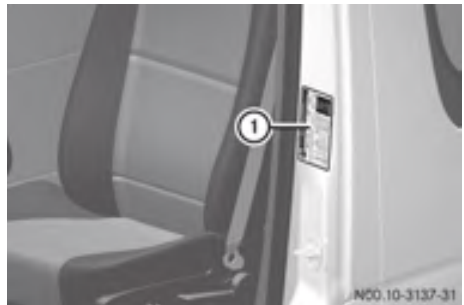
The Tire and Loading Information placard on the driver's door B-pillar
