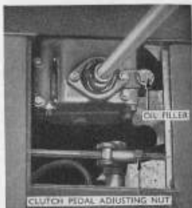
Fig. 26. Access to Change Speed Box and Clutch Pedal Adjuster.
