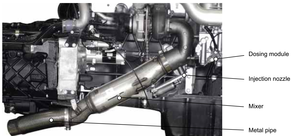
Fig. 46: Exhaust tract, from mixer to metal pipe ESC-426
