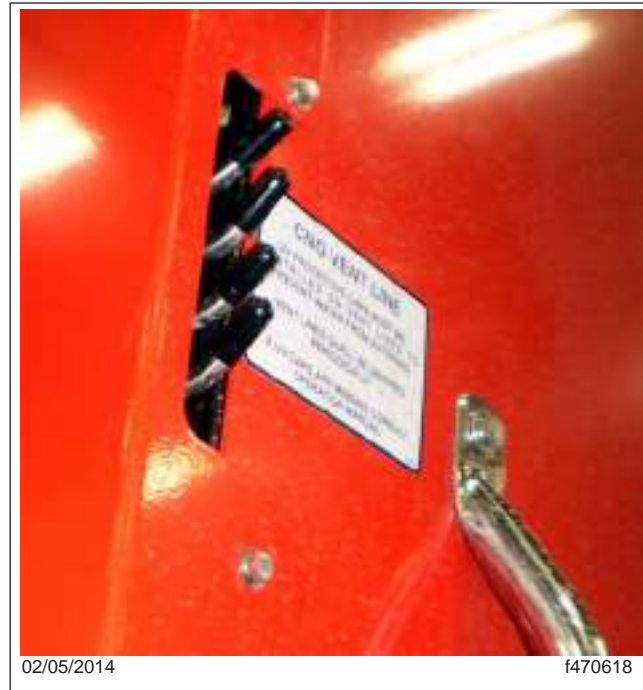
Fig. 21.8, CNG Vent Line Caps
