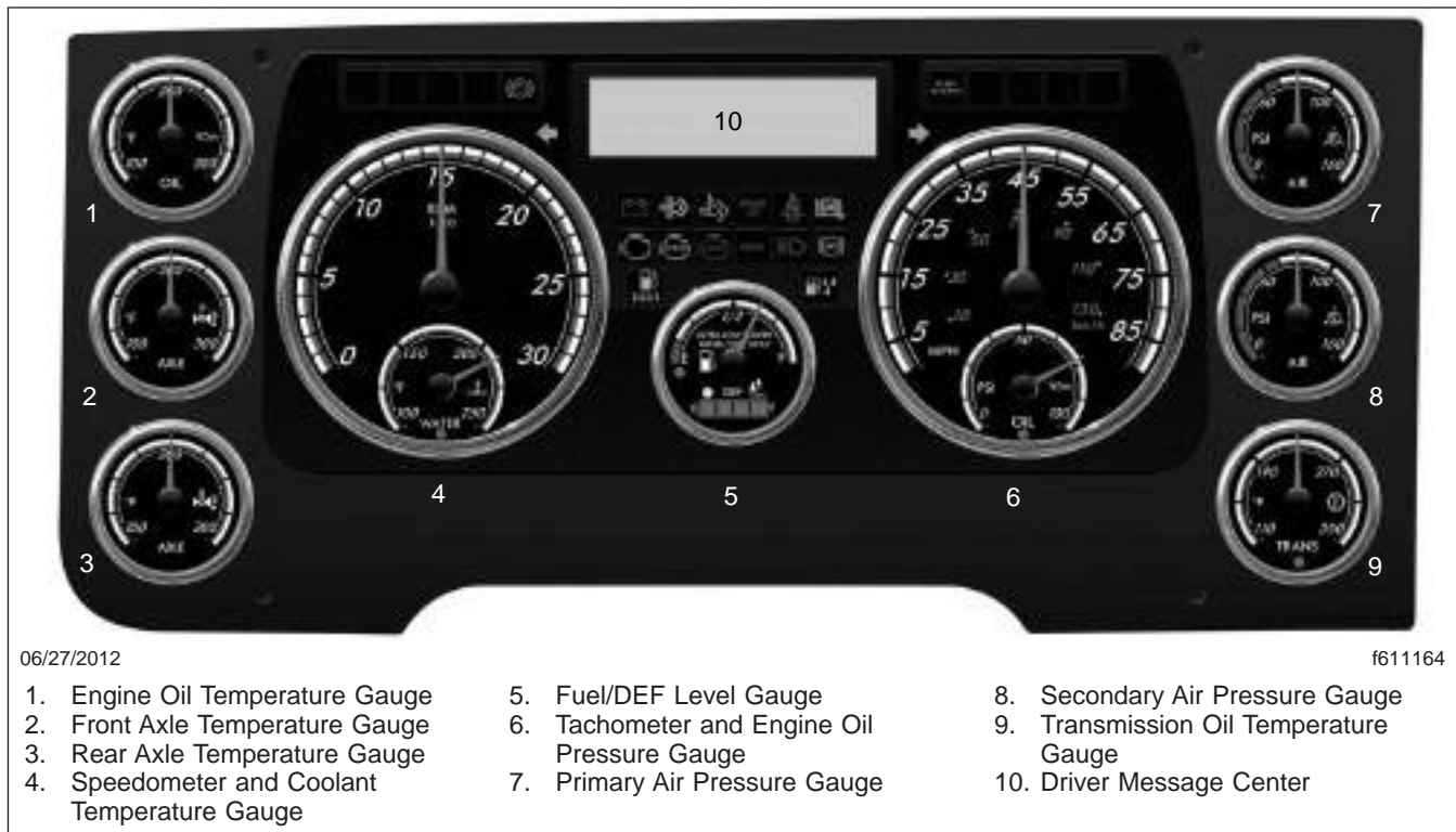
Fig. 4.3, ICU4Me Instrument Cluster
