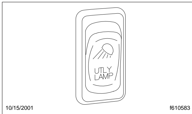
Fig. 4.7, Utility Light Switch
