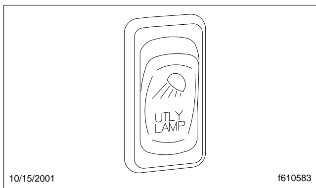
Fig. 5.10, Utility Light Switch
