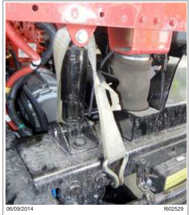
Fig. 24.7, Tension Strap Installed to Hold Down the Cab
