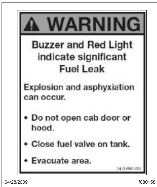
Fig. 19.5, Exterior Warning Sticker
