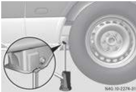
Jacking point, rear axle (example: vehicle type 3500)
