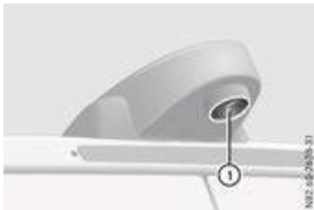
Rear view camera in the middle of the roof above the high-mounted brake lamp
