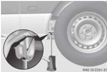
Jacking point, rear axle (example: vehicle type 2500)
