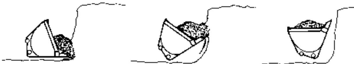
Fig. 4.40. Bank Loading (Working into Material)
