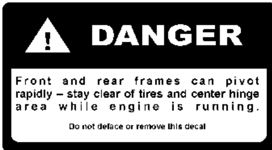
Decal 2 - On the rear frame near the center articulation pivot
