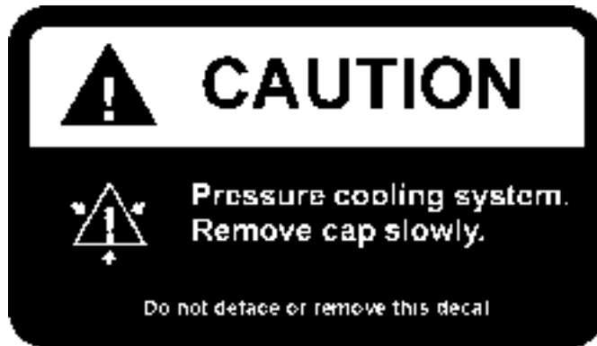
Decal 4 - Near the radiator filler cap
