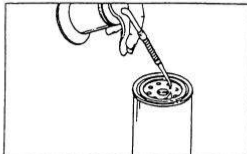
Fig. 5.23. Preparation of Coolant Filter for Replacement
