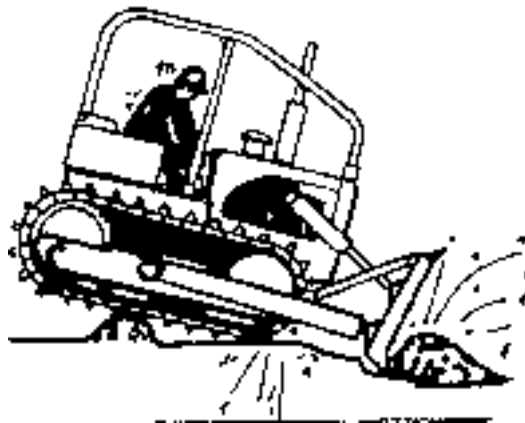
Fig. 4.32. Moving Material Downgrade
