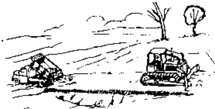
Fig. 4.46. Spreading Material Forward
