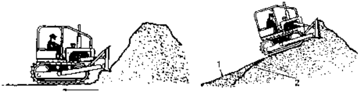
Fig. 4.43. Breaking Down a Pile
