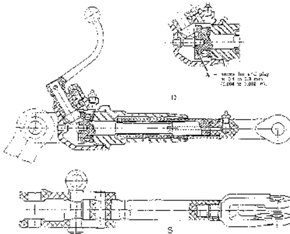
Fig. 191. - Sectional view of the hydraulic lift linkage rods
