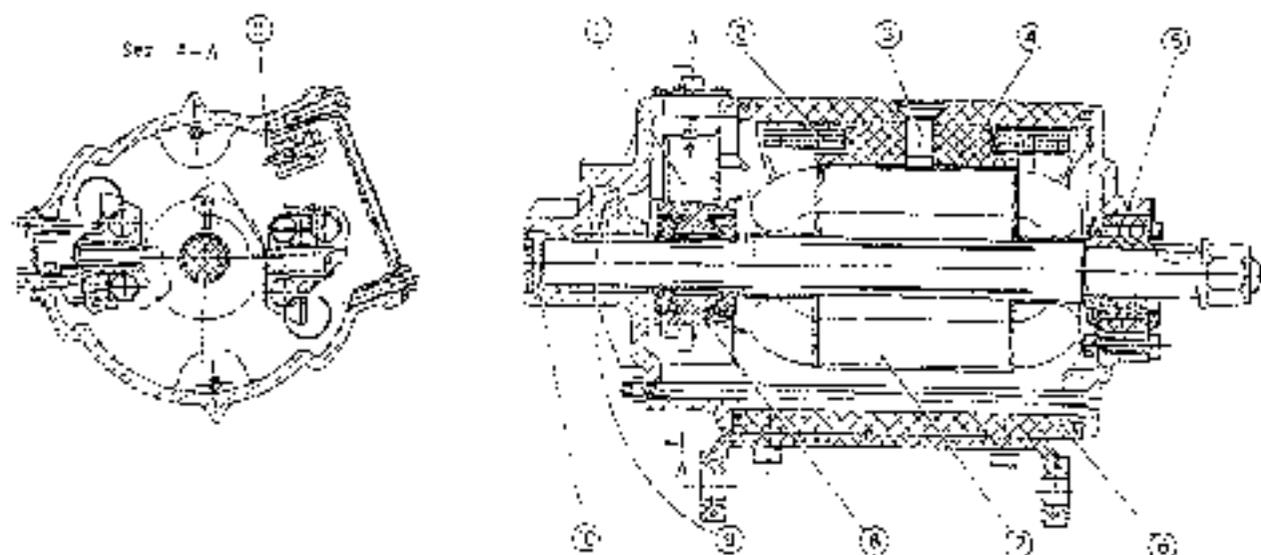
Fig. 128. - Sectional view of generator type R 115-140/24-1600 Var. 2.
