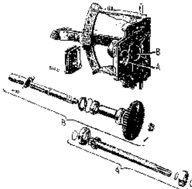
Fig. 168. - Power take-off assembly, stripped.
