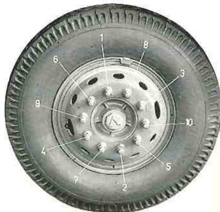
Tightening sequence, disc wheels
