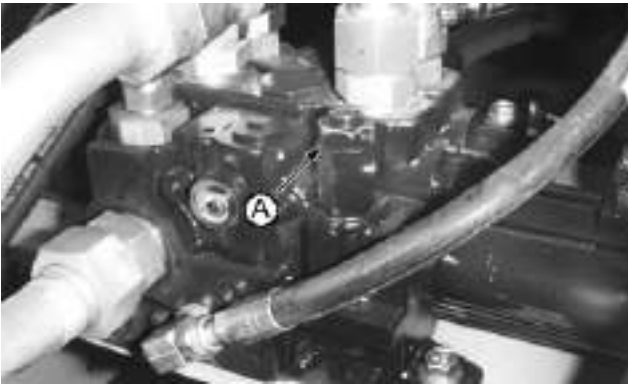
E—Diagnostic Coupler (System Pressure) A—Load Sense Relief Valve—Maximum System Pressure
