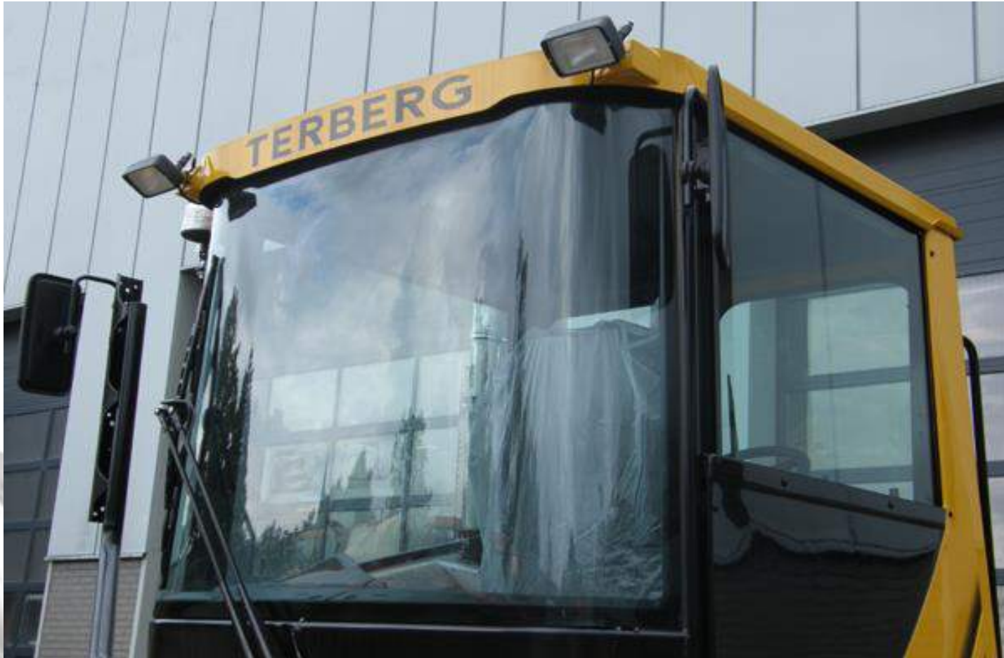
> ROOF LOWERED WITH 120mm
